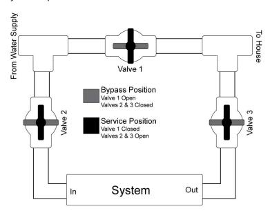
Allow enough room to install a bypass for the filtration system. If something goes wrong with the system, or during maintenance you can still get a water supply to the house. Below is an example of a bypass installation.
