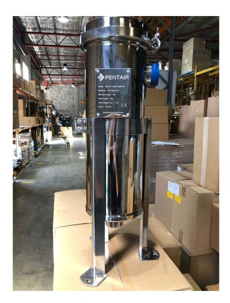
Model BFHC-2-304-2"-BSP-I/O 304 Stainless steel Construction 2" BSP Side In / Bottom Out Ports Band Clamp Closure With Buna Gaskets Maximum Operating Pressure 100 PSI / 690 kPa Operating Temperatures 1°C to 84 °C Takes industry standard #2 filter bags Adjustable Legs
