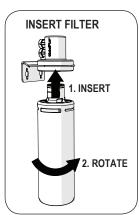
This instruction is for the replacement of the filter in the Zip HydroTap product where the filter is mounted internally. In preparation for your filter flushing, ensure you have a 10 litre container available.
